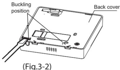
NOTE: Do not pry up and down, you can only rotate the screwdriver.
