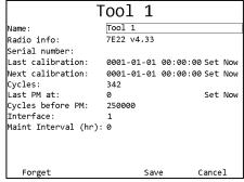
Figure 16: Tool Configuration screen
