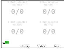
Once loading is completed, the unit should go to the Run screen. If the unit stays on the loading screen with an error, please contact support.
