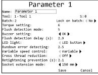
Figure 22: Parameter Edit Screen – AccuPulse
