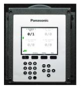
The EYFR04 is equipped with a color LCD display, four soft keys immediately below the LCD, a numeric keypad with decimal point, navigation keys, and enter and escape buttons. The current function of the soft keys is indicated at the bottom of the LCD above the button.
