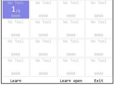
If the tool you are going to learn to the Controller has previously been used with another unit, make sure that unit is off before continuing. Press the button beneath **Learn** to begin the learn process.
