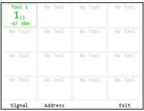
Figure 9: Tool Status - Last signal good
