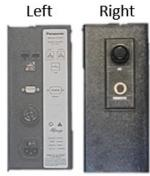
The left side of the EYFR04 has two RJ-45 Ethernet ports to allow it to be used in a chain network configuration.
