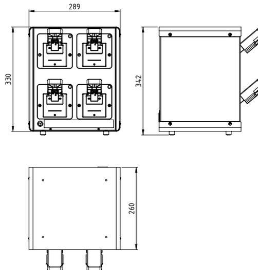
Dimensions in mm (without battery adapter)
