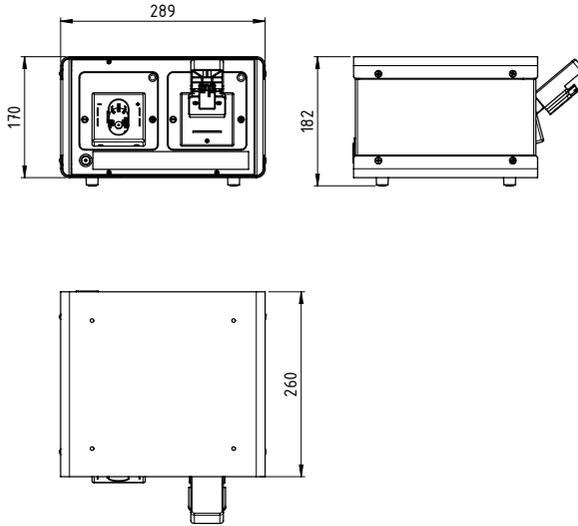
Dimensions in mm (without battery adapter)
