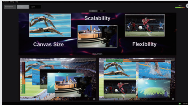
Kairos Creator Live View menu Multi-view videos (MV1/MV2) can be monitored on the GUI software. The image shows an example of a multi-view display that includes 32:9 "Canvas".
