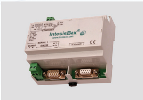
The USPA-AC-BAC-128 is a BACnet over IP server device capable of monitoring and controlling ECOi, ECOi EX and PACi systems. Up to 128 indoor units and 10 refrigerant circuits can be integrated (up to 30 PACi systems). Auto-Discover feature detects connected Panasonic equipment for easy setup and integration. Setup and control via Ethernet port to access GUI.
