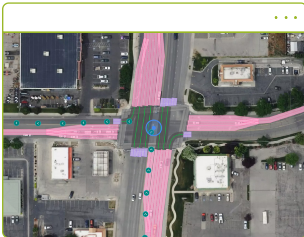
Figure 3: V2X-enabled intersection where a vehicle makes a left turn when the signal appears to not be green, possibly due to the signal showing red in the data but was green at the intersection, or map geometry being outdated, or the vehicle running a red light. Note: green lines indicate the signal is green and absence of a line between intersections indicates that the signal is red.
